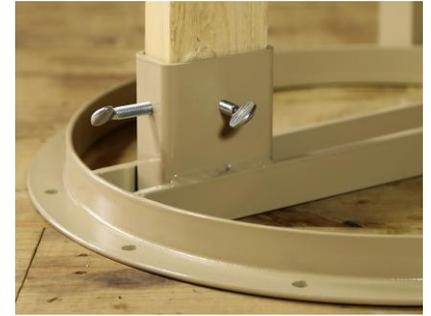
Have your local wood supply store cut 2x4 lumber down to 3 feet in length. Note that 2x4 lumber is an actual size of 1.5 inches by 3.5 inches. This size **MUST** be used to properly fit into the base. Apply adequate pressure by tightening the thumb screws that are already installed in the base. They are found on the back and side of the base.
