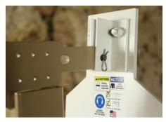
Place top bracket onto the top of the 2x4 upright. The angles shown on the back of the target will already be installed on your target. All you have to do is slide the top bracket between the angles as shown, then lining up the holes, slide the clevis pin through to the other side. Be SURE the pin is through before letting go of the target plate.
