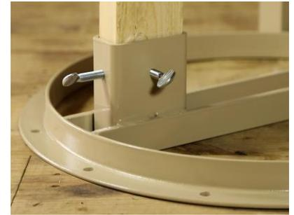
Have your local wood supply store cut 2x4 lumber down to 4 feet in length. Note that 2x4 lumber is an actual size of 1.5 inches by 3.5 inches. This size **MUST** be used to properly fit into the base. Apply adequate pressure by tightening the thumb screws that are already installed in the base. They are found on the back and side of the base.
