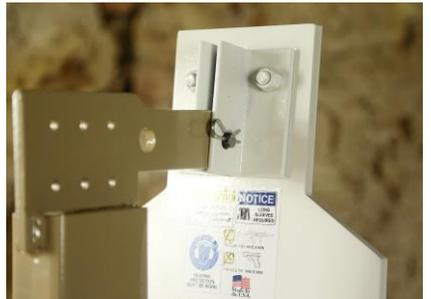
Place top bracket onto the top of the 2x4 upright. The angles shown on the back of the target will already be installed on your target. All you have to do is slide the top bracket between the angles as shown, then lining up the holes, slide the clevis pin through to the other side. Be **SURE** the pin is through before letting go of the target plate.
